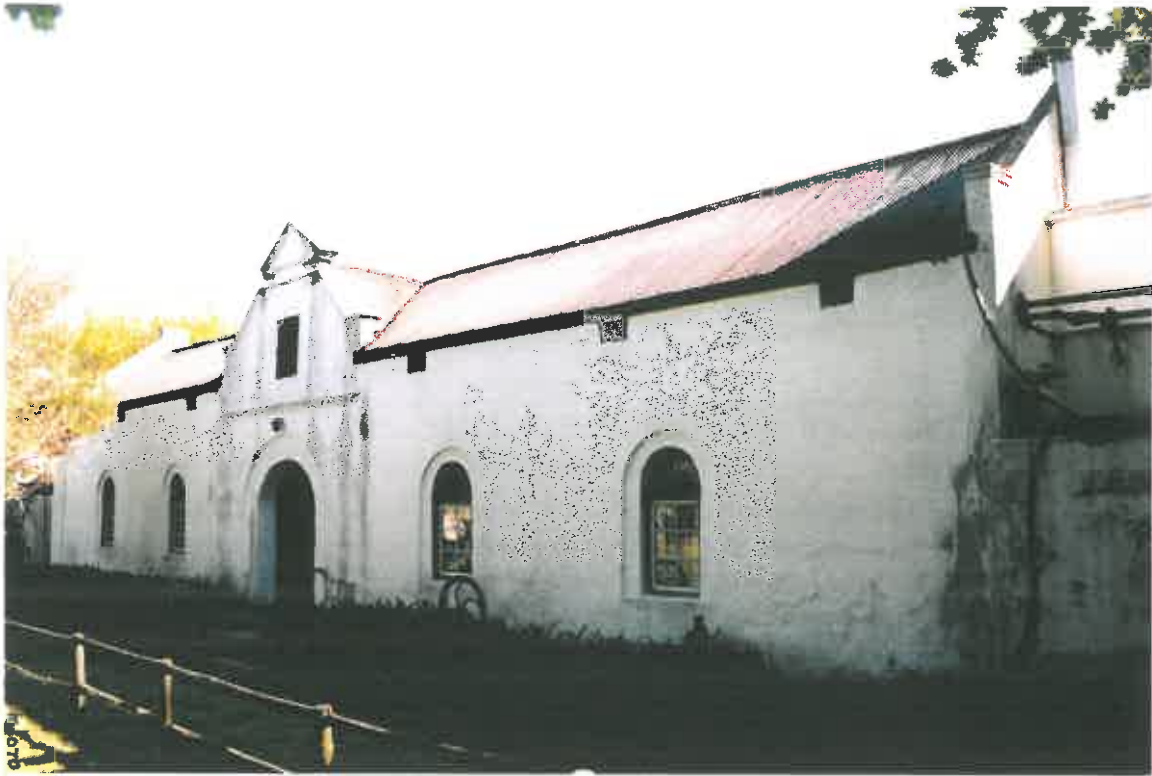
7. During the height of wine exports, a neo-classical wine-cellar was erected by Frans Roussouw in c.1820. The windows were fixed with iron spokes in the upper segments as a security measure.
